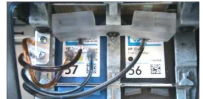
Visible Ink Levels & Detachable tanks
